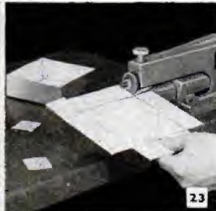
Straight cuts can be made freehand by following a pencil line, but a better way is to improvise a guide as in left-hand photo. Center photo shows how notches are cut to form box corners. Right-hand photo shows how a curved guide can be used to form a true radius. In this case, an ordinary washer served the purpose
